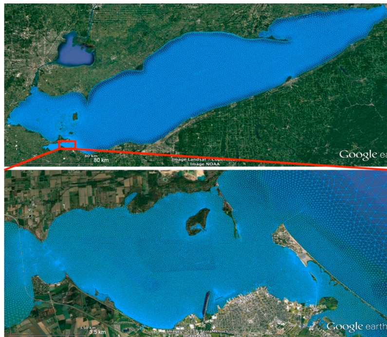
Figure 3. Finite volume community ocean model (FVCOM) model mesh for Lake Erie ( upper panel ) and linked with a high-resolution mesh for Sandusky Bay ( lower panel ). Only a portion of the Sandusky Bay mesh is displayed for a clear representation of the mesh’s resolution.
