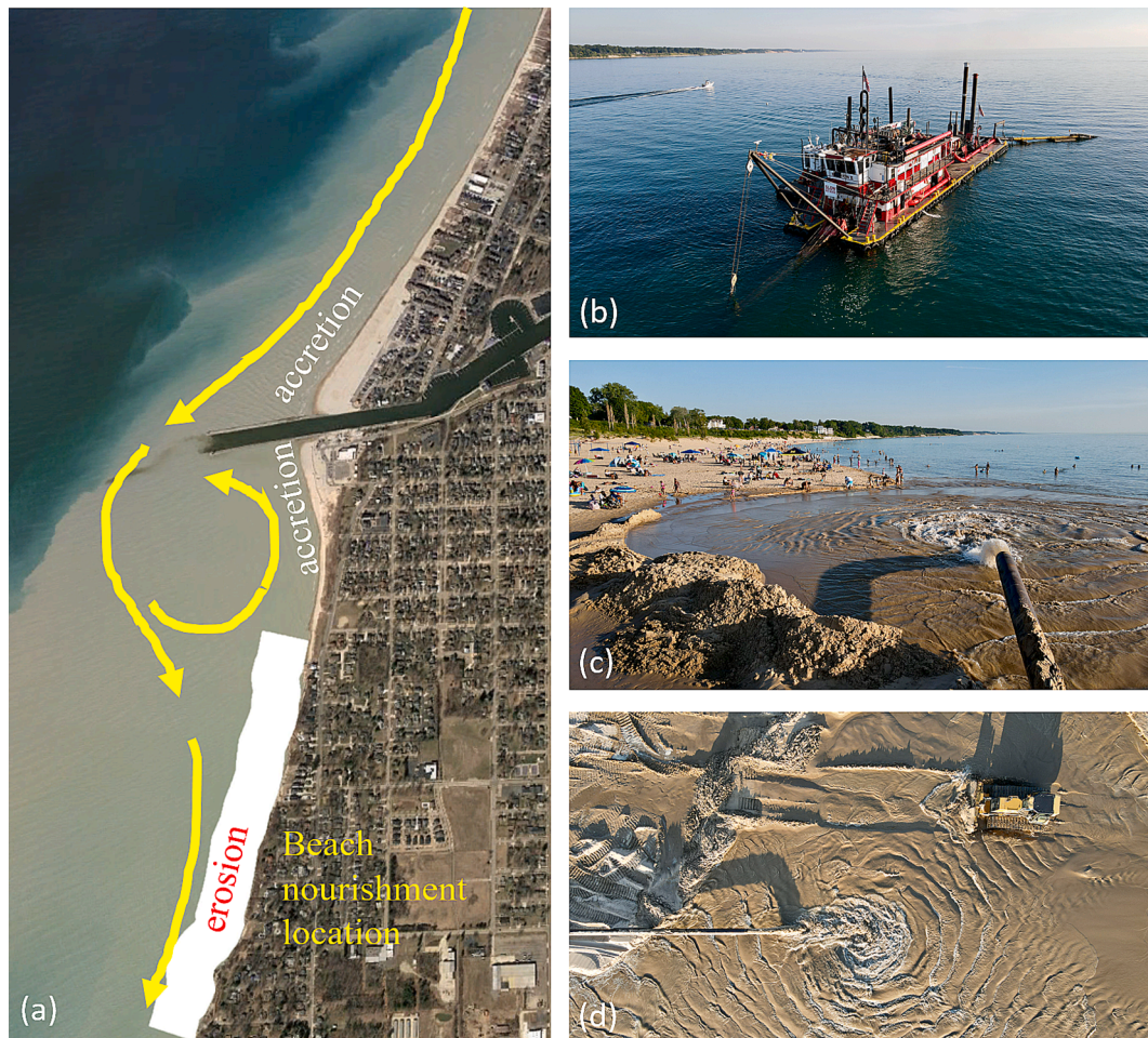
Fig. 14. (a) Sketch for the sediment accretion and erosion near the jetty, where the arrows indicate the dominant direction of the currents (as well as the sediment transport) in storm time and the white area indicates the location for the beach nourishment by U.S. Army Corps of Engineers in August 2022 ( https://www.lrd.usace.army.mil/Media/News-Releases/Article/3132077/corps-of-engineers-to-begin-dredging-beach-nourishment-in-south-haven/ ). (b-d) Beach nourishment on the South Beach in South Haven in June 2023. (b) A hydraulic dredging platform. (c) and (d) Beach nourishment. Photo. Source: https://www.mlive.com/public-interest/2023/06/beachgoers-frolic-around-south-haven-harbor-dredging-outwash.html
